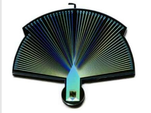
Figure 3.6: Close-up photograph of the PEACOQ detector which can detect photons at a rate of a gigahertz.<sup>128</sup>
