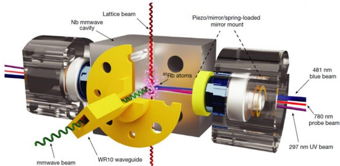
Demonstrated at U. Chicago and Stanford, with QLCI HQAN. Rydberg atoms in superconducting and optical cavities convert microwave to visible photon states.
